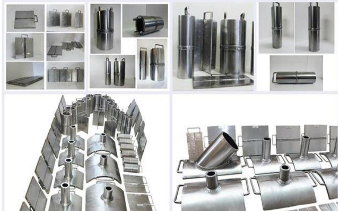
Flawed Specimen Test Components
